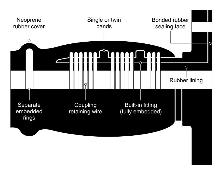
Built-in rubber lined (fully embedded) coupling system (for A20 dredge hose)
