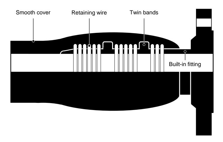
Built-in (full-bore) coupling system (for oil delivery hose)
