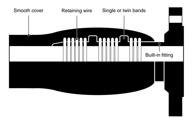
Built-in (full-bore) coupling system (for delivery hose)
