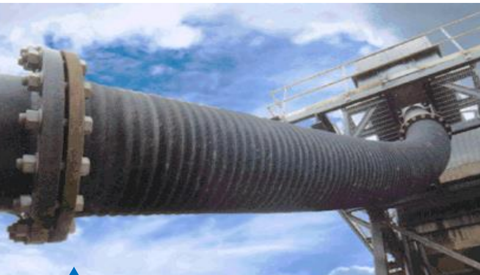
A113 gravel and rock hose with beaded end swivel flanges
